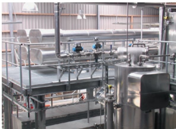
Figure 8: TDH unit for thermal pretreatment from ATZ (photo and unit by ATZ, Germany).
