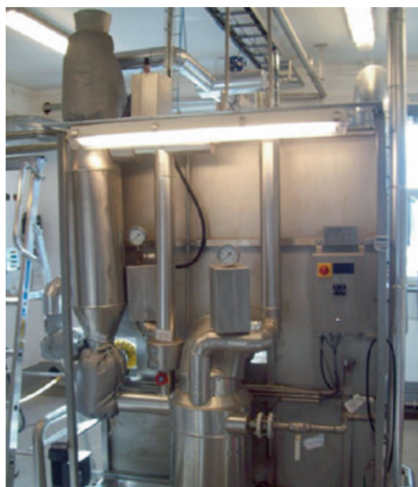
Figure 9: Pilot-scale steam explosion unit by CAMBI, Norway (photo by University of Natural Resources and Life Sciences, Vienna, Division of Agricultural Engineering).
