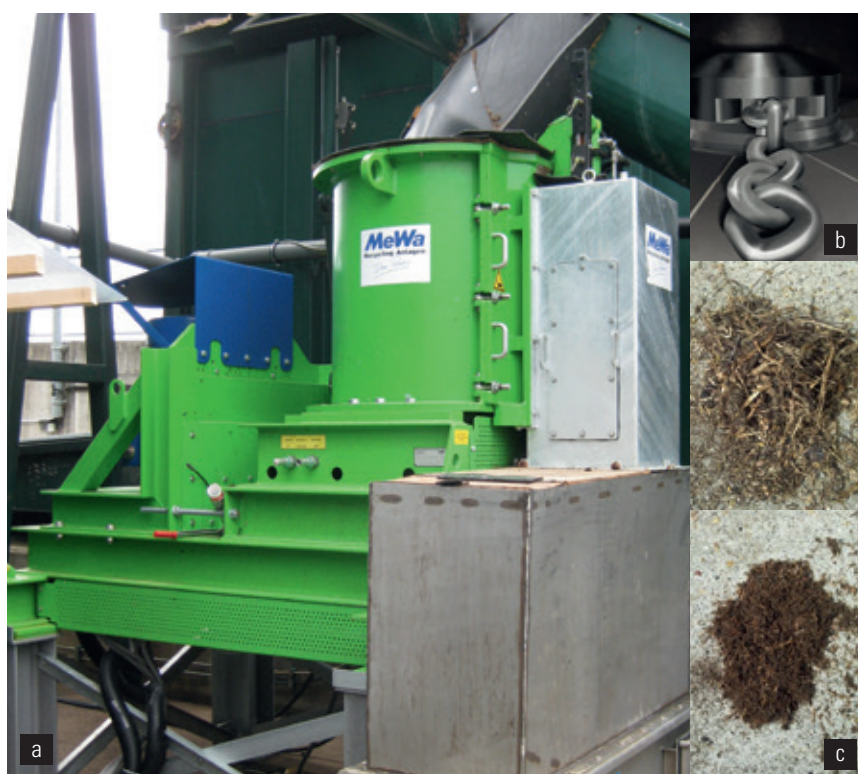
Figure 7: Example of a mechanical pretreatment unit called “Querstrommerspanner” (sometimes called cross-flow shredder) by MeWa Recycling Maschinen und Anlagenbau GmbH, Germany (a). Inside the chamber of the machine, a thick metal chain (b) spins around and the impact of the chain on the fibres causes them to break (cutting and grinding). This unit is installed at an agricultural biogas plant using grass silage as a main substrate. Unmilled (left), partially milled (middle) and fully milled grass silage (right) (images a and c by Siegfried Legath, image b from ANDRITZ Mewa).
