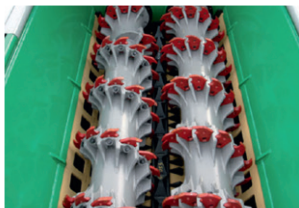
Figure 5: Example of a shredder called CRAMBO by Komptech GmbH, Austria (image from Komptech).
